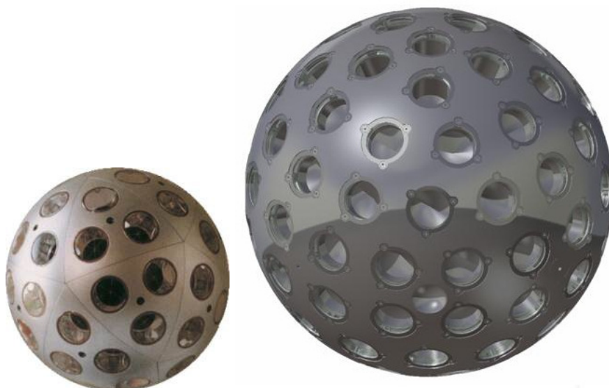
Fig. 1 Starlette (left) and LARES (right). The proportion of the scale is kept. Left: http://wwwrc.obs-azur.fr/gemini/themes/geo/satellites/ . Right: http://www.lares-mission.com/ .
