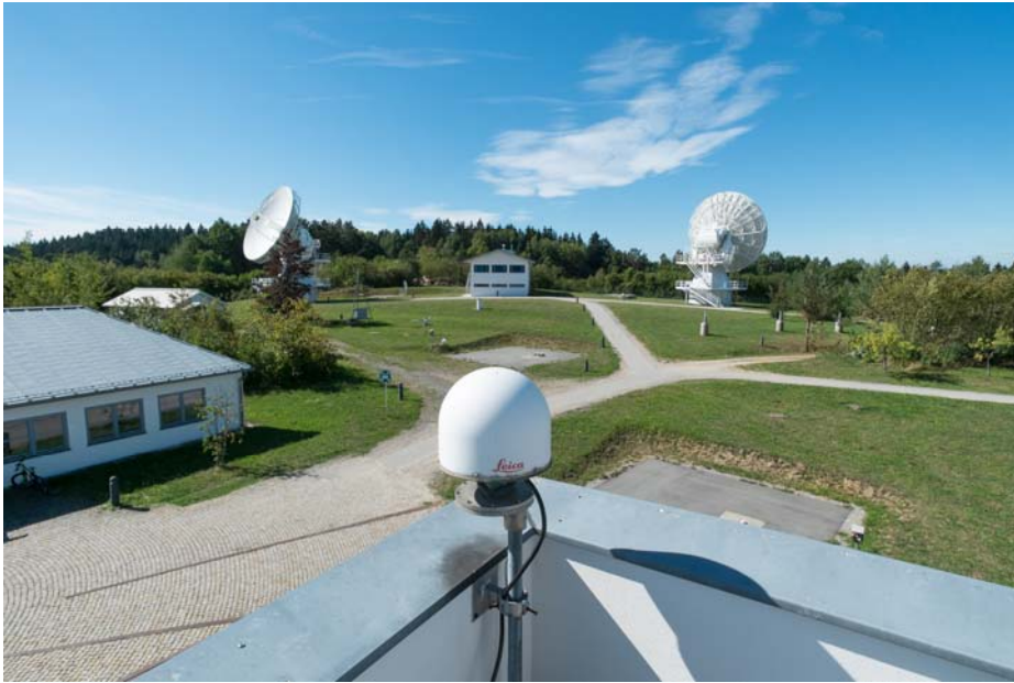
Fig. 1: Antenna of the GNSS station WTZR (Wettzell, Germany). The photo was provided by Uwe Hessels from the Federal Agency for Cartography and Geodesy.
