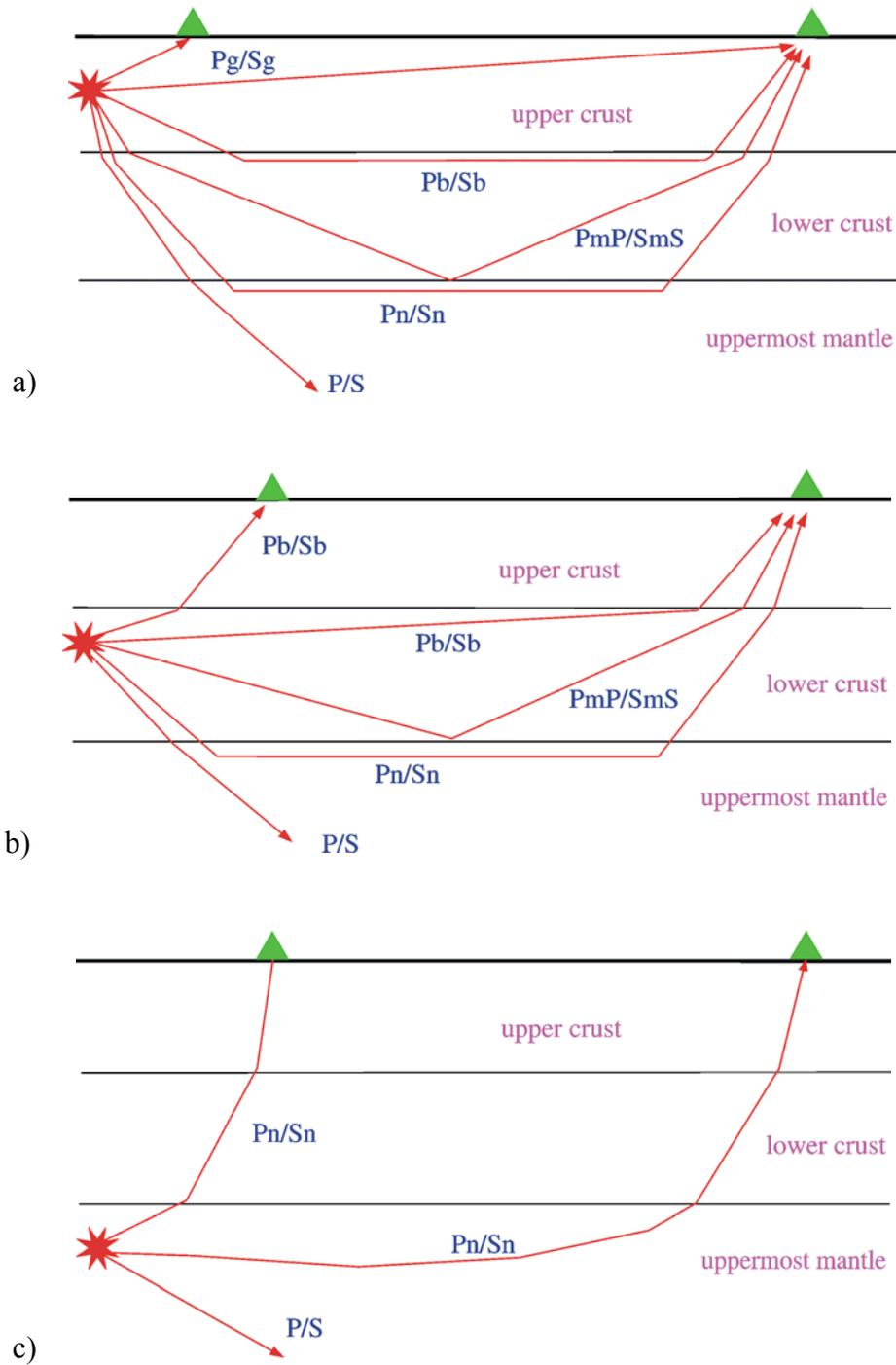
**Figure 1** Seismic rays of „crustal phases“ observed in the case of a two-layer crust in local and regional distance ranges ( $0^\circ < D < \text{about } 20^\circ$ ) from the seismic source in the: a) upper crust; b) lower crust; and c) uppermost mantle.
