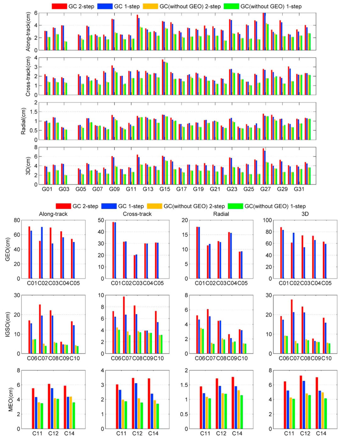
Figure 10. Average root-mean-square of GPS and BDS orbit overlap differences for GC combined precise orbit determination with 34 global stations. GEO = Geostationary Earth Orbit; IGSO = Inclined Geosynchronous Satellite Orbit; MEO = Medium Earth Orbit.
