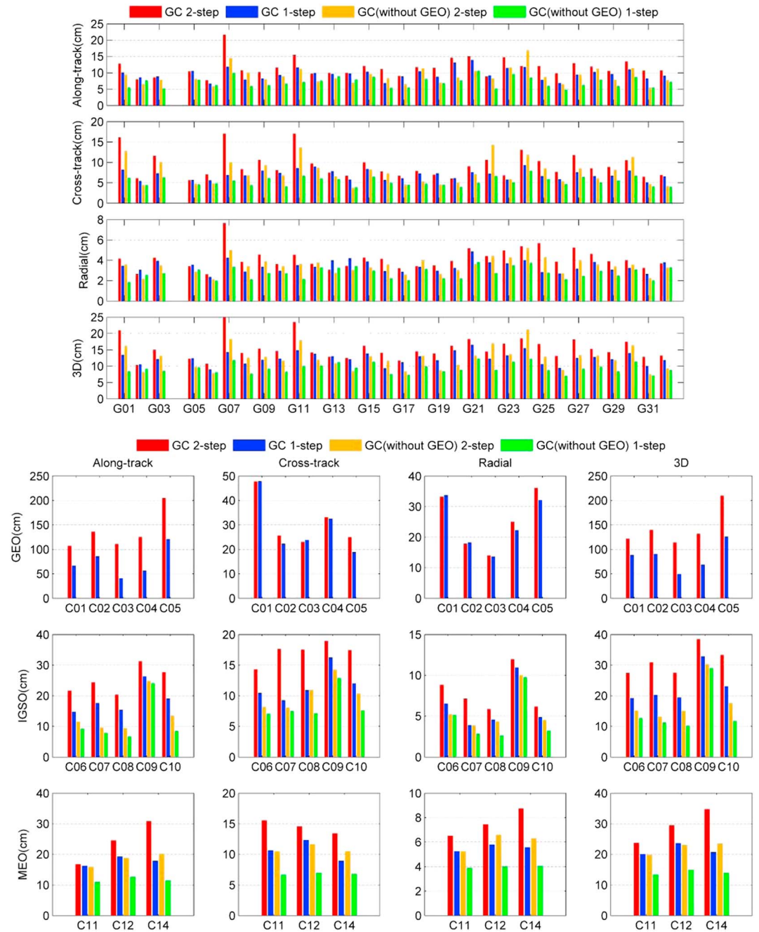
Figure 6. Average root-mean-square of GPS and BDS orbit overlap differences for GC combined precise orbit determination with 10 regional stations. GEO = Geostationary Earth Orbit; IGSO = Inclined Geosynchronous Satellite Orbit; MEO = Medium Earth Orbit.
