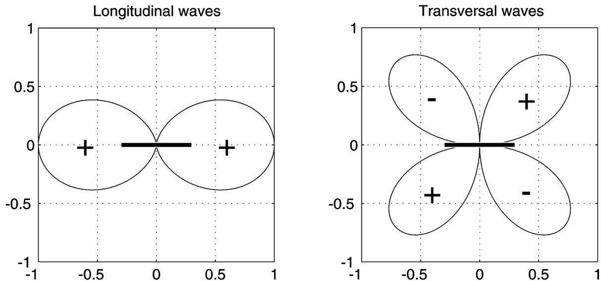
**Figure 3** Relative direction sensitivity of linear strainmeters to apparent longitudinal (left) and apparent transversal (right) elastic waves. The strainmeter is indicated by the thick horizontal bar in the center of diagrams. Note that in both cases the strainmeter response is identical for opposite arrival directions.
