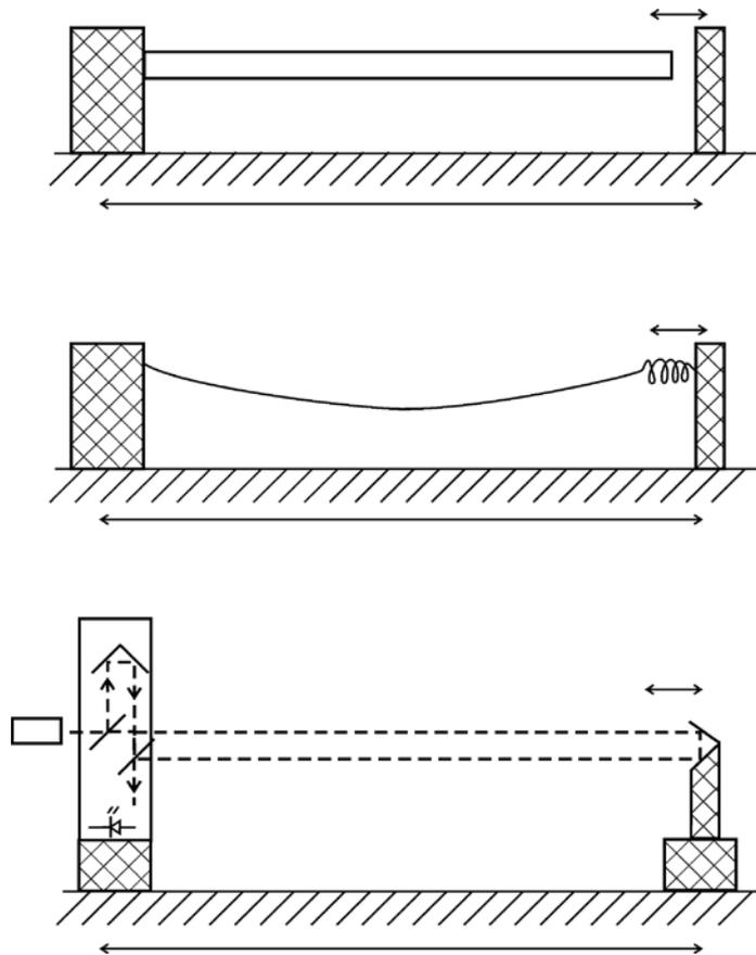
**Figure 1** Schematics of the most frequent strainmeter designs. From top to bottom: rod-, (tensioned) wire- and laser strainmeters. The top two must be equipped with displacement transducers at the right. The bottom sketch indicates the laser, two beam splitters, one corner cube reflector and some sensor (symbol of photodiode) able to detect the change in the interference fringes due to the relative motion of the corner cube reflector on the pedestal to the right.
