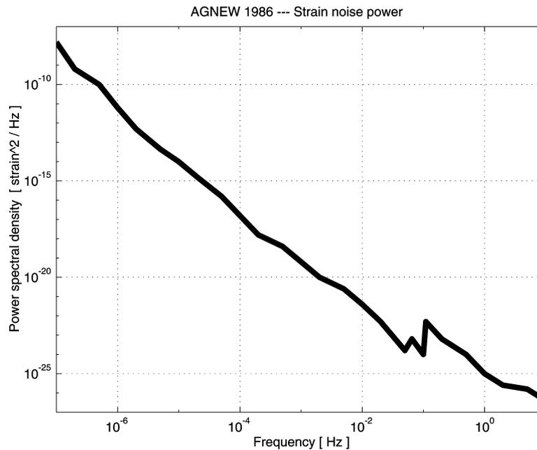
**Figure 2** Power spectral density in (strain squared)/Hz as published by Agnew (1986). This is from the 730 m-NW laser horizontal strainmeter at Pinion Flat, California. This instrument is installed at the surface, but referenced with "optical anchors" to a depth of 30 m (Wyatt et al. 1982). See discussion of noise sources in text.
