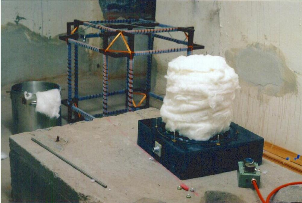
**Figure 2** Some kind of synthetic wool, polyester stuffing, or fleece material is gently wrapped around the seismometer. The gap between the gabbro plate and the casing of the instrument is also filled with fleece to prevent air convection. Be careful to keep the thermal insulation loosely fitting. The fleece must not exert forces on the seismometer casing.
