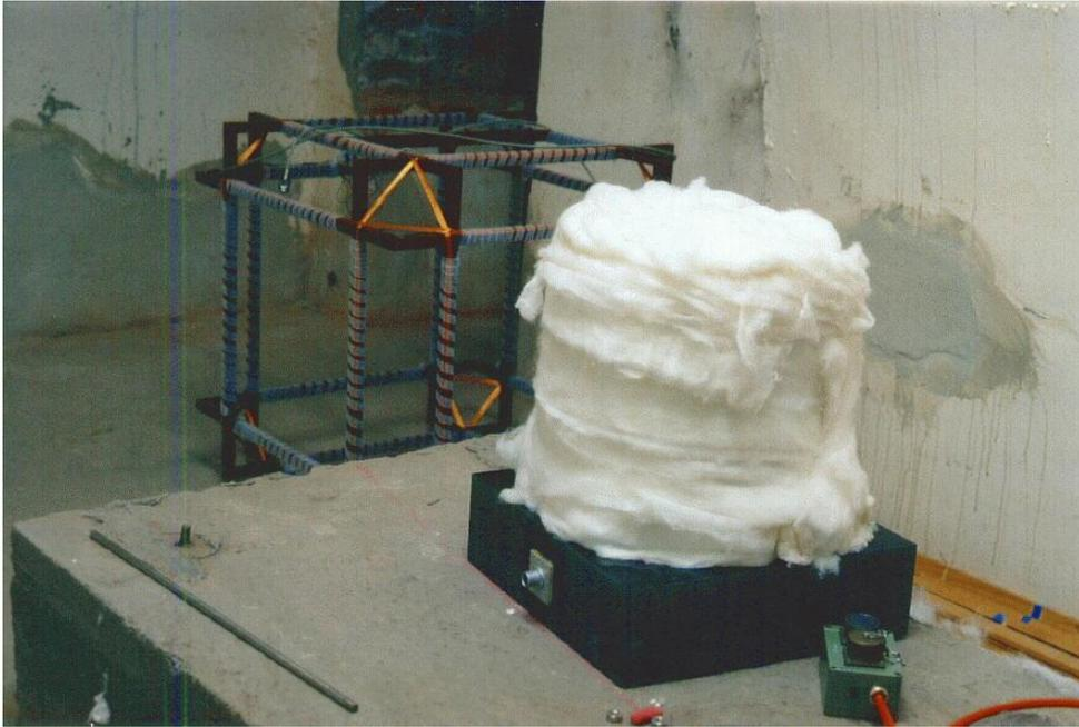
**Figure 4** A second layer of stuffing or fleece is wrapped around the steel container. Other than in this picture it is recommendable to wrap the gabbro plate too. The fleece again serves as a thermal insulation and prevents air drafts from acting directly on the surface of the instrument. Synthetic stuffing fleece with stronger fibres is preferable for this outer layer. The stronger fibres are able to maintain the structure of the fleece even when exposed to high humidity.
