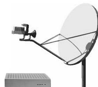
Figure 11 Example of a VSAT modem (indoor unit) and parabolic antenna with receive and transmit unit (outdoor unit).
