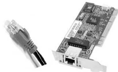
Figure 4 Example of an RJ45 connector and a PCI based network interface card.
