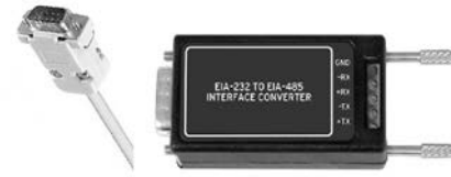
Figure 3 Example of an RS-232 to RS-485 adaptor.
