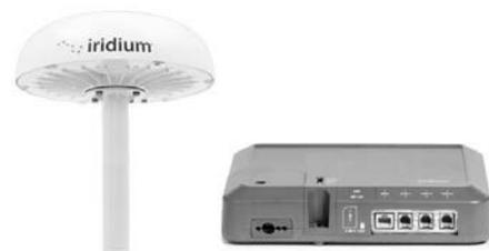
**Figure 17** Iridium antenna (ADE) and OpenPort terminal (BDE).
