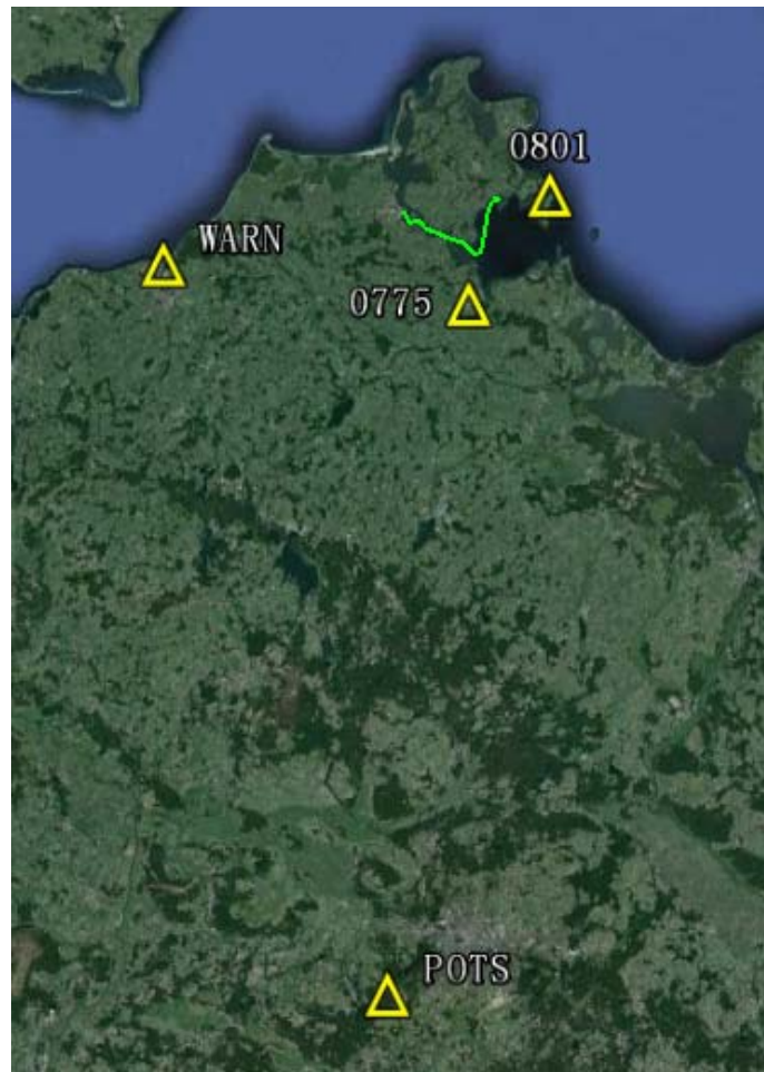
Figure 5.4: The track of the ship (green curve) and the positions of reference stations (yellow triangles) for the Baltic Sea shipborne gravimetric experiment on June 18, 2013
