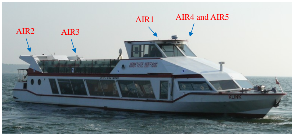
Figure 8.3: The ship used and the position of GNSS receiving equipments
