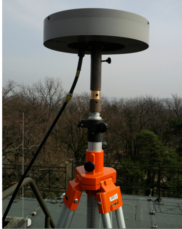
Figure 3.3: Equipment for the vertical movement experiment of a GNSS antenna
