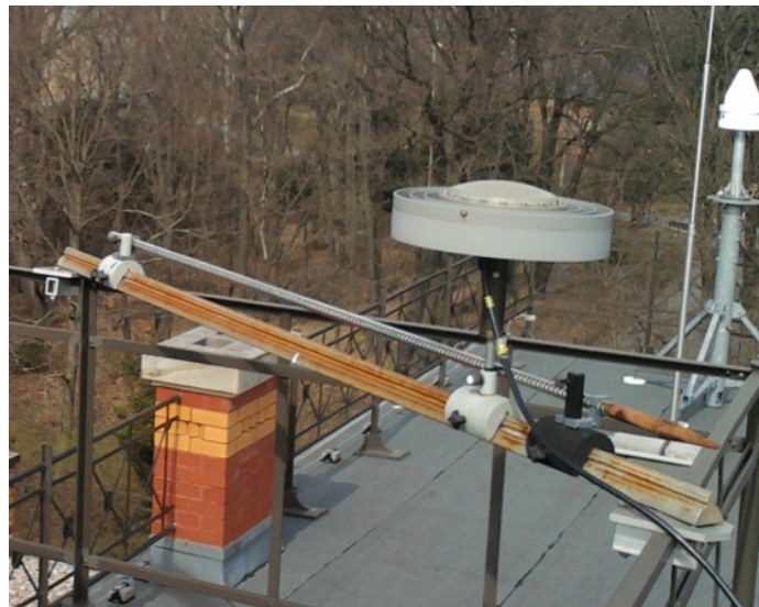
Figure 3.2: Equipment for the horizontal movement experiment of a GNSS antenna
