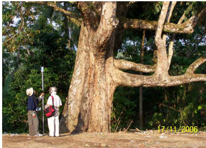
Figure 2.20 Example of the 2006 survey at station M21, showing manually using of the ENVI PRO. One operator has to handle the equipment (hold the sensor and carry the console) and read the measured values, while the other has to write the readings on the data sheet, immediately. These data then have to be inputted to the computer manually for data processing.
