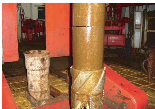
Figure 7. Torsional failure of the bit sub during Expedition 309. A horizontal gash opened for ~150° (11 inches) of the circumference of the 3/4-inch thick bit sub wall, ~15 inches from the bit, with more ragged fracture tips propagating a further ~75° around the pipe from each end of the clean fracture. When in tension with the drill bit hanging from the sub, the fracture opened up to 1 cm, and the bit was held on by only ~4.25 inches of the bit sub wall.
