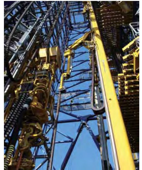
Figure 3. High powered top drive and pipe handling system, setting a 4-stand drilling pipe to the pipe racker.
