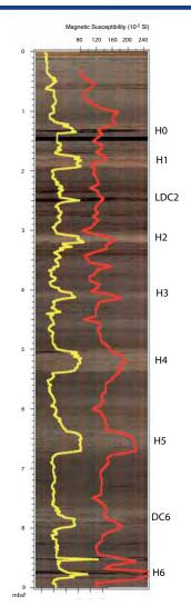
Figure 2. Detrital layers at Hole U1303B, in the uppermost 9 mbsf. Enhanced digital image scan overlain by susceptibility (red, right) and gamma ray attenuation density (yellow, left). Detrital layer nomenclature from Stoner et al. (2000) for Core MD95-2024 taken nearby.
