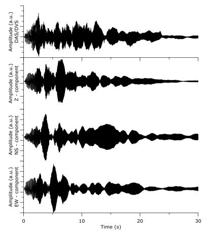
Figure 3: Comparison of measured signal from the optical fiber buried in a 50 cm deep trench (top) below a three component geophone (three traces at the bottom).
