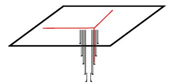
Figure 1: Conceptional design of the fiber-optic installation within the IMAGE project (not to scale). The cable (red) will be installed down to a depth of 1200 m. Some additional cable length shall be deployed at the surface to create a three dimensional sensor array.
