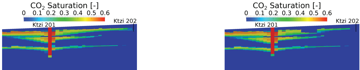
Fig. 4. Dumux model: Section through Ktzi 201 and Ktzi 202: CO 2 plume expansion after 255 days for Cases 2 and 2b-b2. The barrier feature can be detected as a blue rectangular spot in the right upper region of the right-hand figure.
