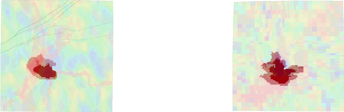
Fig. 6. Permeability field (log scale) and CO 2 plume for mid of October 2009 (dark red) and 2012 (light red); Approach I left, Approach II right.
