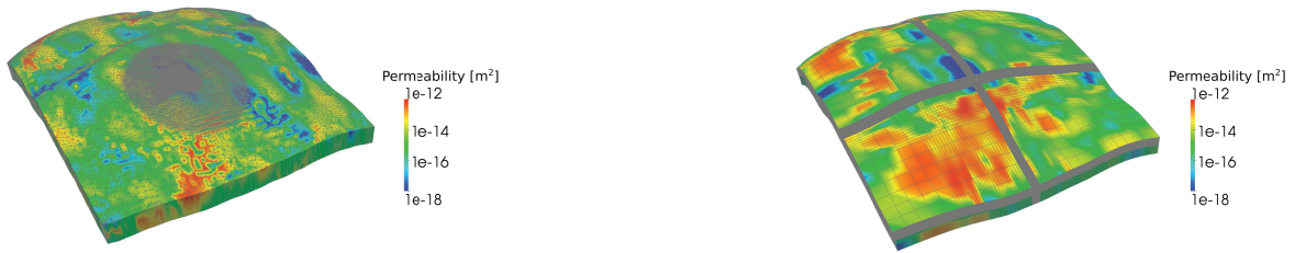
Fig. 1. Tetrahedron (left) and hexahedron mesh (right) with interpolated permeability fields (five times vertically exaggerated).
