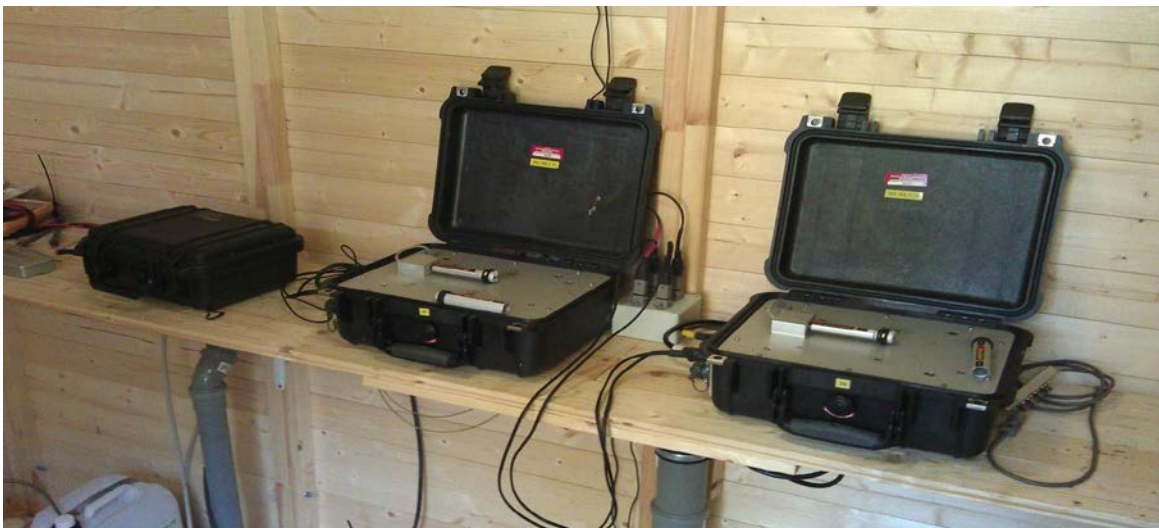
Fig. 4: Inside the wooden hut - data are recorded with GPS-synchronized S.P.A.M. Mk IV data loggers.
