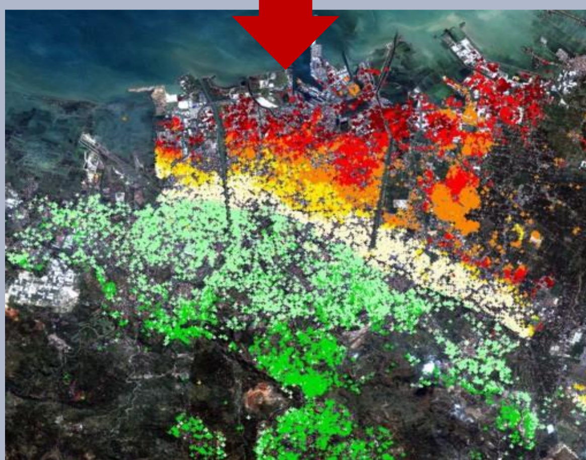
PS-points with classified annual motion rates over section of IKONOS MS satellite image of Semarang taken on May 22, 2005 © BGR, Germany (Includes material ©2002, Space Imaging LLC.)
