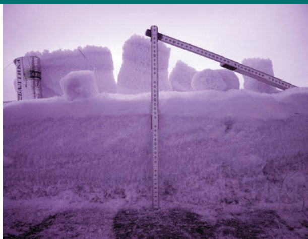
Infrared photography of a snow profile: the lower 3/4 of the snowpack consists of large depth hoar crystals, which are efficient insulators (Martin Proksch).
