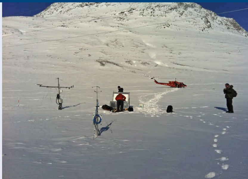
Figure 7. Tower measuring exchanges of carbon dioxide between the land surface and atmosphere (Torben R. Christensen).
