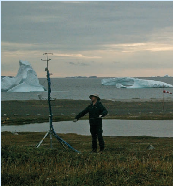
Instrument mast with high-resolution wind measurements and air intake for trace gas analyses set up near the Arctic Station (Disko Island, Greenland) (Thomas Holst).
