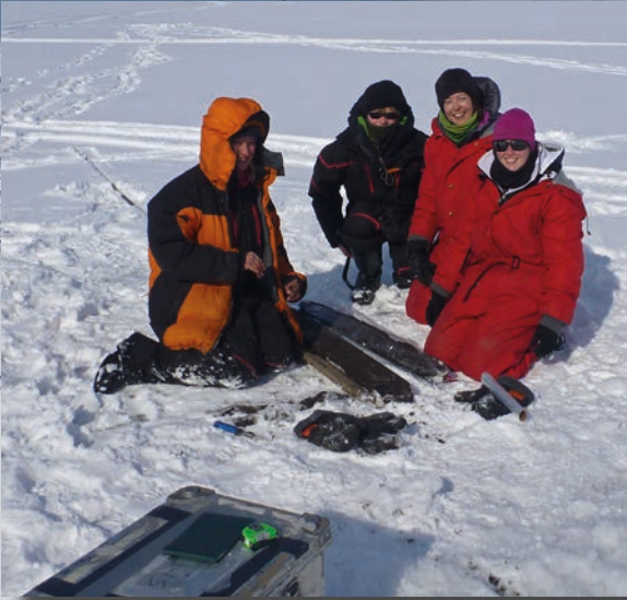
We used a Russian corer which is attached to rods (visible in the photo above). A video of the coring can be seen on www.youtube.com/watch?v=Q7Yc-ok2dAs#t=53 (Suzanne McGowan).
