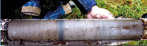
Saksunarvatn ash layer (the visible dark-coloured tephra layer is 2 cm thick) from a sediment core (K.J. Edwards).
