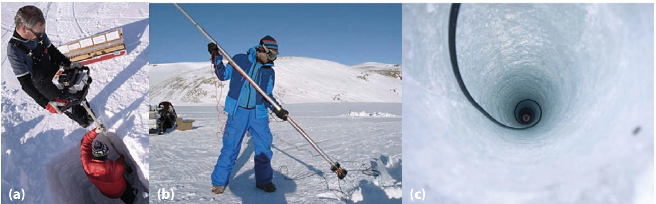
Drilling of a borehole and deployment of a seismic sensor (S. Mertl (a), G. Weys (b), D. Binder (c)).
