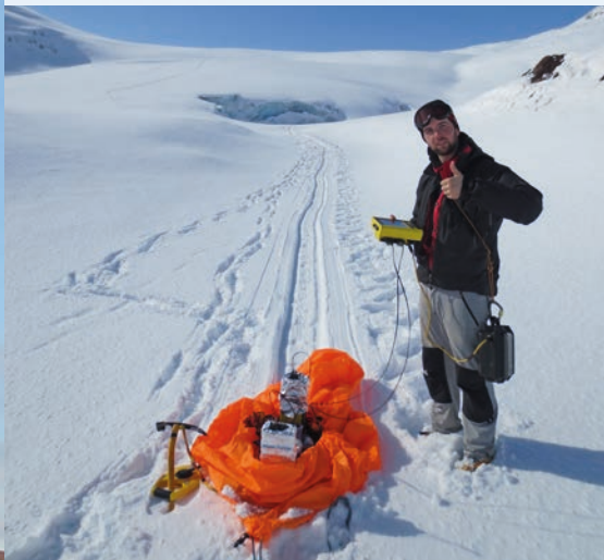
The GPR being used in front of the glacier snout during winter. The transect along which the survey has been taken can be seen behind the GPR. The photograph has been taken looking east (Kathryn Adamson).
