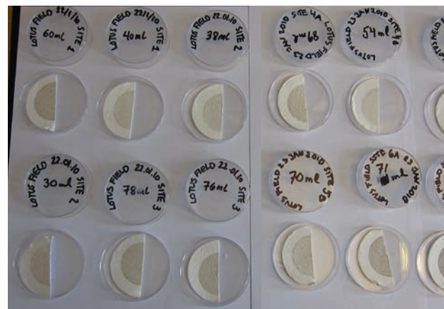
Filters for the Thermo/Optical Carbon Aerosol Analyzer (filters are cut in two). These are samples taken in 2010 from Changbai, Northeast China. You can clearly see the dark half circle where the meltwater including tiny black carbon particles has darkened the filter (Christina A. Pedersen).
