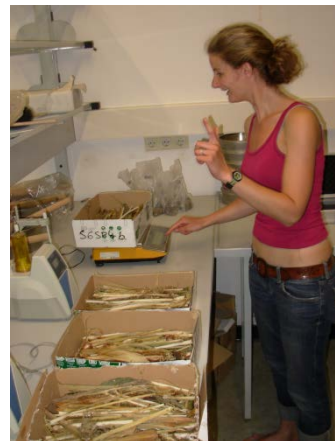
Figure 6.14: After drying, the samples were taken from the oven (left) and the dry mass was determined on a laboratory scale (right).
