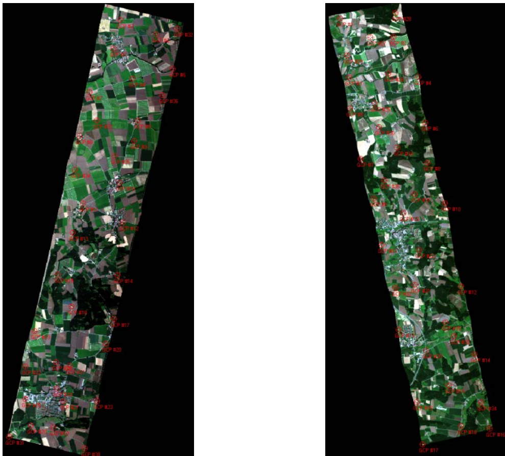
Figure 3.03: Geometric processing of both HyMap acquisitions using GCPs and a 1 st order polynomial nearest neighbour transformation in ERDAS 9.3 (Neusling: left, Steinbeißen: right).
