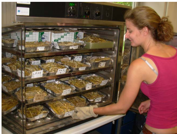
Figure 6.14: After drying, the samples were taken from the oven (left) and the dry mass was determined on a laboratory scale (right).
