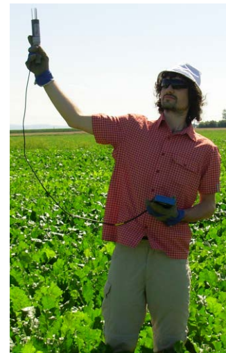
Figure 6.21: ThetaProbe ML2x (User Manual, page 3, left) and student assistant Mr. Jochen Scholtes, calibrating the ThetaProbe in the middle of a sugar beet field (right).
