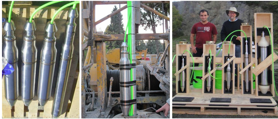
Fig. 3 Left the first GONAF station instrumentation at Tuzla borehole. Right the optimized array after the Tuzla test from left to right three levels of 1 Hz vertical L-4s, a combined 2 and 15 Hz 3-C, and
