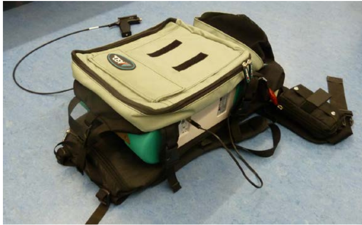
Figure 2-5: ASD FieldSpec 4 kept in the backpack; equipped with several storage pockets, a battery and a pistol grip for accurate fixation of the fiber optic cable.
