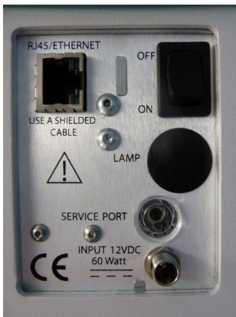
Figure 2-3: Console for technical controls and connections at the back of the FS4.
