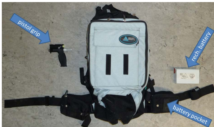
Figure 2-2: ASD FieldSpec 4 kept in the backpack; equipped with several storage pockets, a battery and a pistol grip for accurate fixation of the fiber optic cable.
