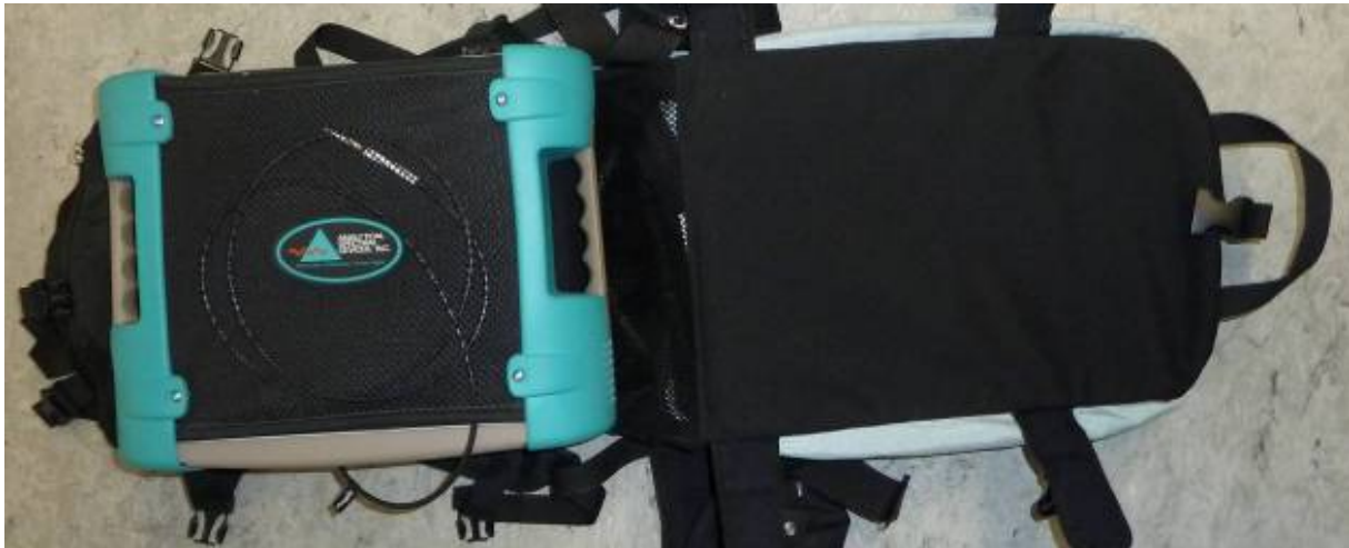
Figure 2-1: ASD FieldSpec 4 in an open backpack with the fiber optic cable curled and safely stored.
