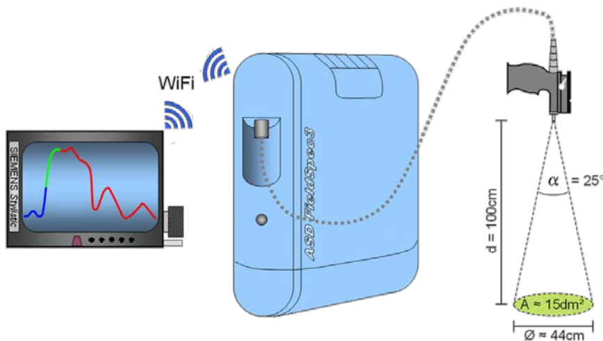
Figure 2-6: Schematic illustration of the technical arrangement of a hyperspectral field- or laboratory measurement.
