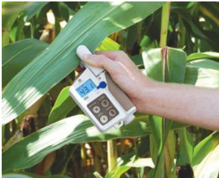
Figure 2-3: Example for measuring with SPAD-502plus.
