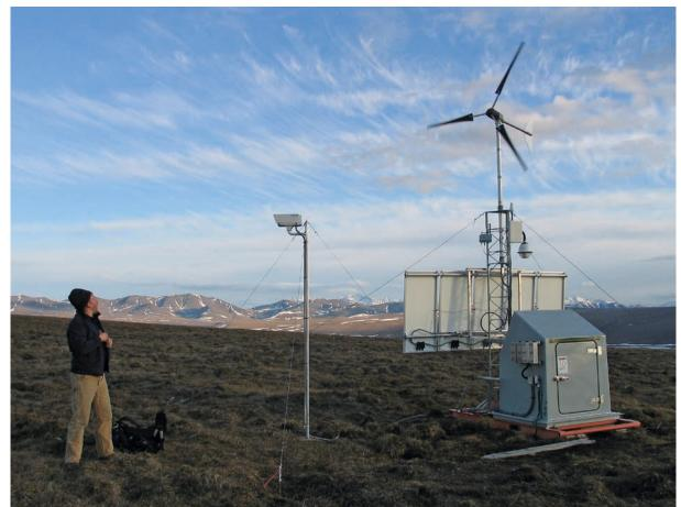
Wind power can be used as power supply for remotely located instruments (Elmer Topp-Jørgensen/Aarhus University).
