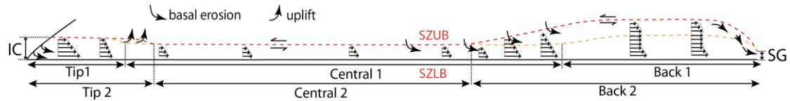
Figure 5.1.2. Main characteristics of the SC, based on the close up image of the SC in figure 5.1.1v. The SC is confined by upper and lower continuous active shear zones (SZUB and SZLB). Arrows illustrate magnitude and sense of displacement of single particles inside the SC. The lateral differences of the vector velocity field define its Tip, Central and Back segments. The length and width of the SC segments were transient over time, here illustrated with Tip1, Central1 and Back1 during a first step of convergence and Tip2, Central2 and Back2 during a second step of convergence. The upper boundary of the Back segment additionally underwent an upward migration due to the migration of the faster particles (also see Figs. 5.1.4b and c). The transverse velocity gradient behaves as that of a channel flow (the velocity at the bottom is the largest, as adjoins that of the conveyor belt and decreases upward until reaching its lowest value at the top). Basal erosion occurs along the contact with the Central and Back segments but is the strongest where the SC widens, i.e. the frontal part of the Back segment (see also figure 5.1.4b; see Section 5.1.5).
