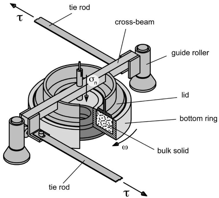
Fig. 4. Ring-shear tester (after Schulze, 1994).
