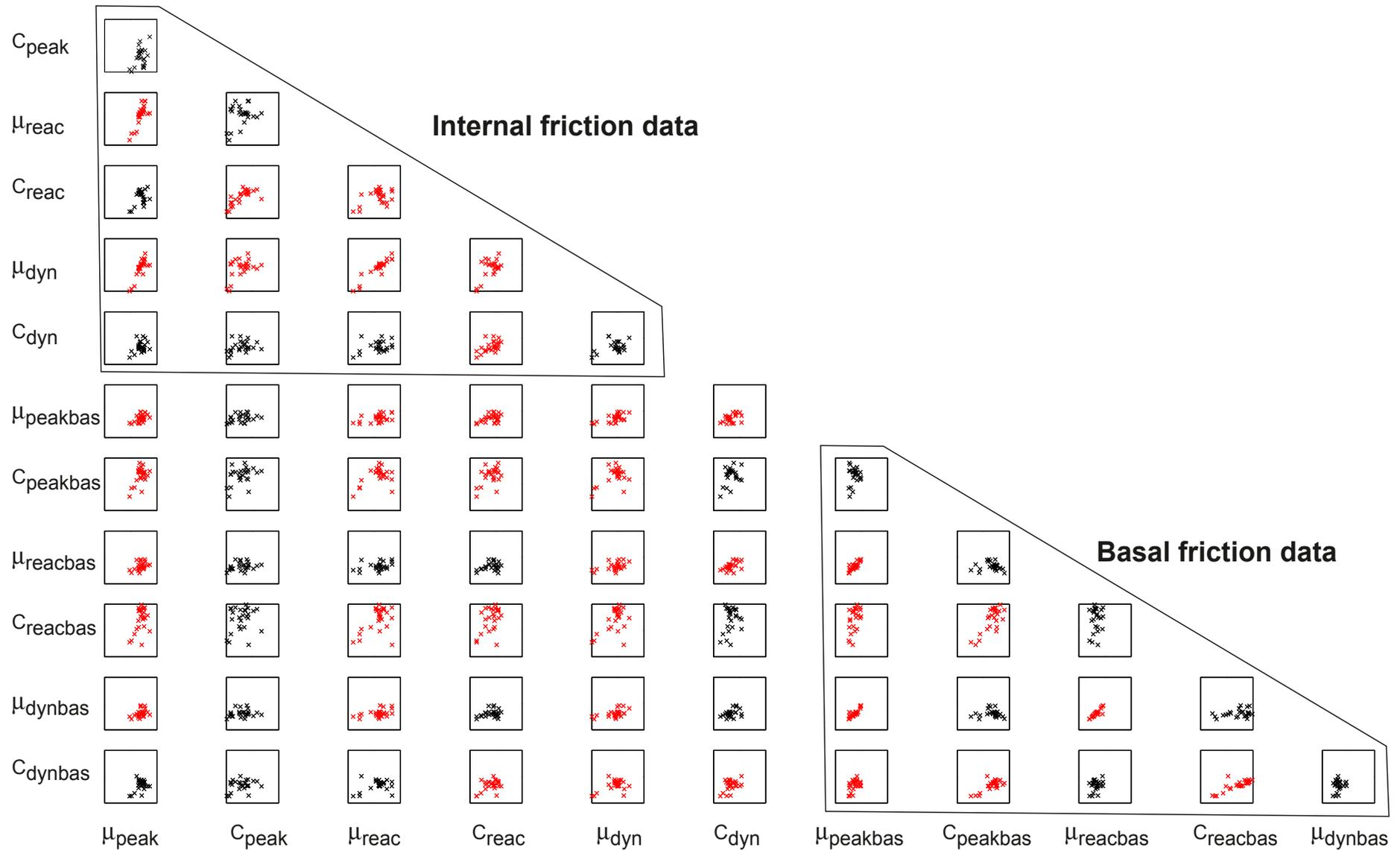
Appendix 1. Bivariate cross-correlation matrix of internal and basal friction data. C is cohesion,  $\mu$  is coefficient of friction; subscripts “peak”, “reac” and “dyn” indicate respective values at internal peak, internal reactivation and internal dynamic conditions, respectively; subscripts “peakbas”, “reacbas” and “dynbas” indicate respective values at basal peak, basal reactivation and basal dynamic conditions, respectively.
