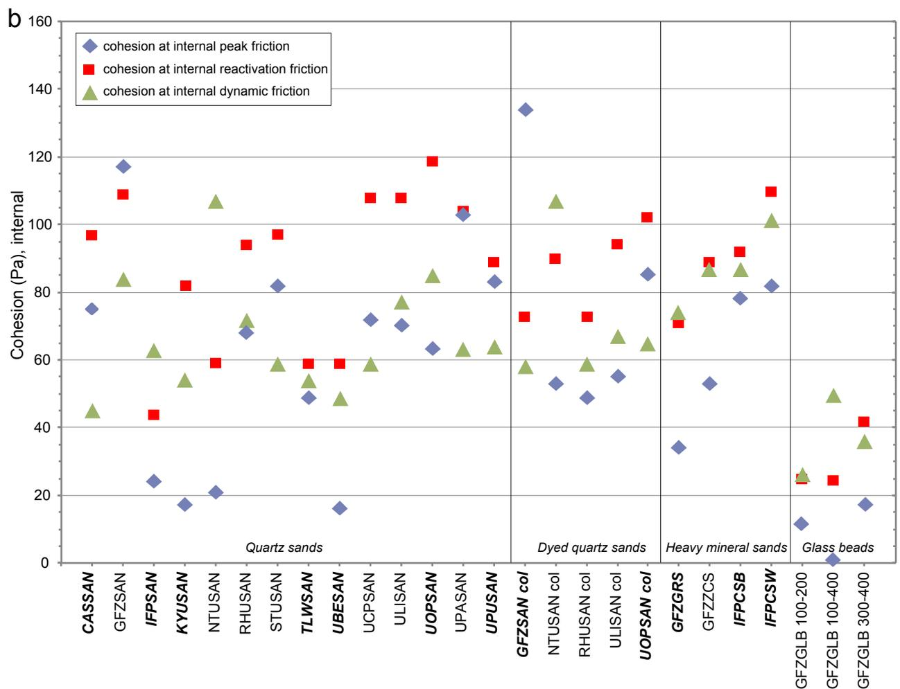
Fig. 8. Internal friction angles and cohesion values (a) Angles of internal peak friction, internal reactivation friction and internal dynamic friction. (b) Extrapolated cohesion values at internal peak friction, internal reactivation friction and internal dynamic friction. Angular granular materials are indicated in bold italics, rounded materials in normal font.
