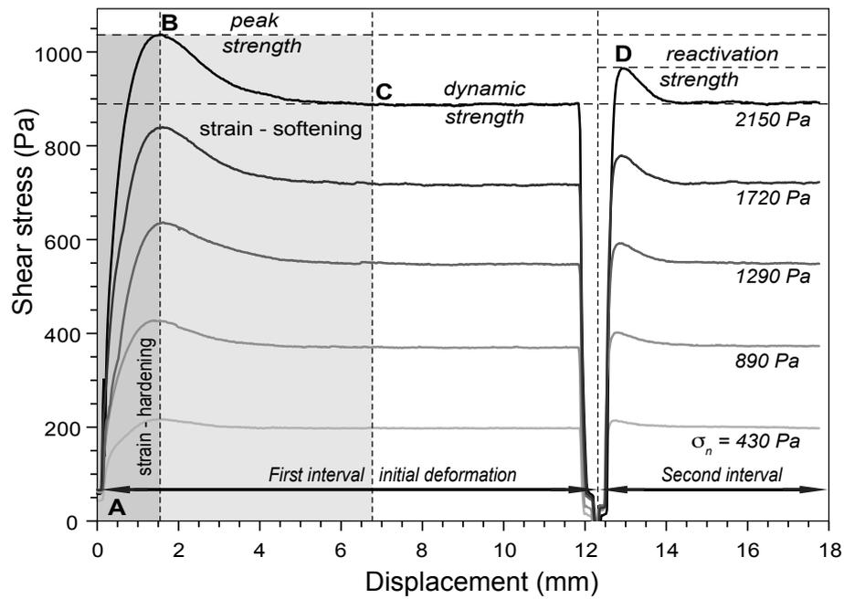
Fig. 5. Example of shear stress curves at different normal loads, AB = strain hardening part of curve, BC = strain softening part of curve, B = peak strength, C = dynamic strength, and D = reactivation strength.
