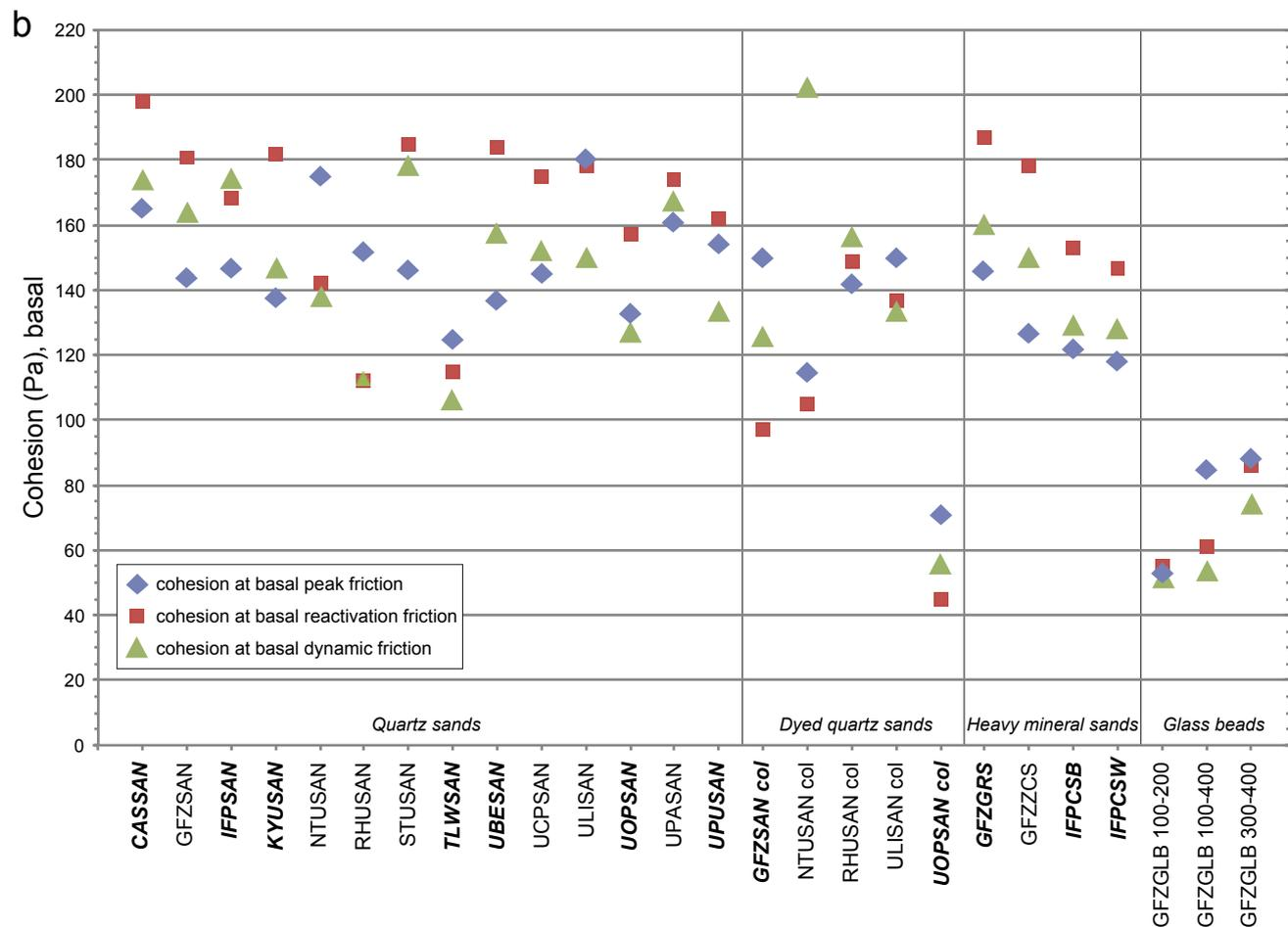
Fig. 9. Basal friction angles and cohesion values (a) Angles of basal peak friction, basal re-activation friction and basal dynamic friction. (b) Extrapolated cohesion values at basal peak friction, basal reactivation friction and basal dynamic friction. Angular granular materials are indicated in bold italics, rounded materials in normal font.
