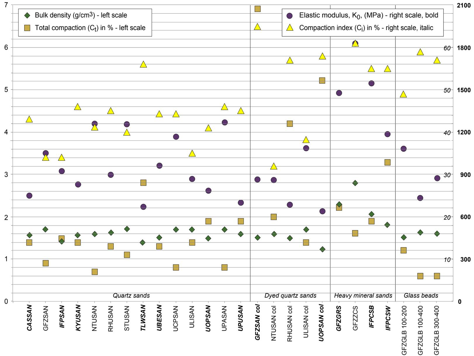
Fig. 11. Values of bulk density, compaction index (left scale), total compaction and elastic modulus, K<sub>0</sub>, (right scale). Angular granular materials are indicated in bold italics, rounded materials
