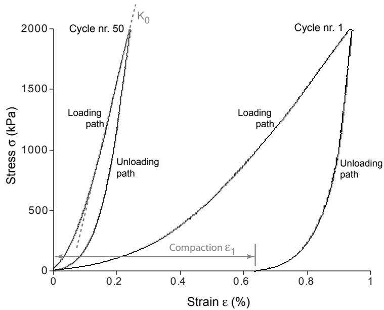
Fig. 10. Uniaxial confined compression test after the first and 50th cycle. First loading – unloading cycle is dominated by compaction; later cycles represent more elastic behaviour. The elastic modulus,  $K_0$ , is determined at the 50th cycle along loading path (dashed line).
