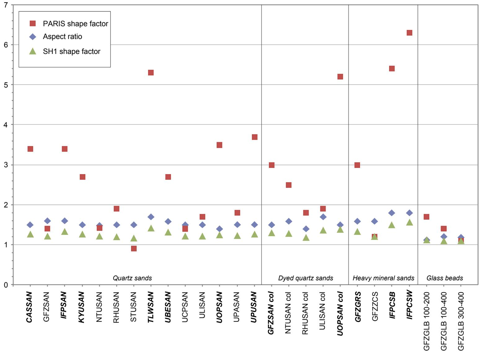
Fig. 3. Grain shape analysis using aspect ratio, and SH1 shape and PARIS factors. Angular granular materials are indicated in bold italics, rounded materials in normal font.
