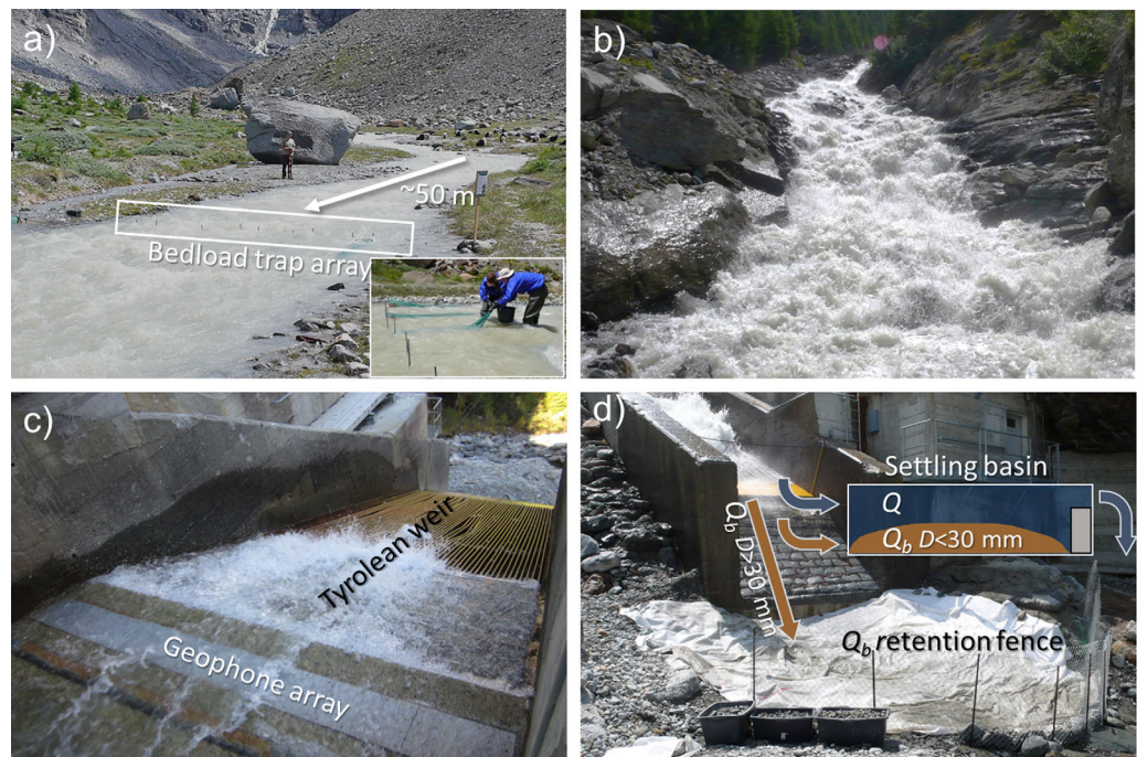
Figure 1. (a) Bed load transport study reach on the low-gradient glacier forefield with S=0.028 \text{ m m}^{-1} and a bankfull width of about 6.8 m. The inset shows researchers emptying the bed load traps. (b) Steep study reach with S=0.38 \text{ m m}^{-1} and a bankfull width of about 5.9 m. (c) Water intake downstream of the steep study reach, showing the Swiss plate geophone array and the Tyrolean weir that separates the coarse bed load from the water. (d) Coarse bed load Q_b with D>30 \text{ mm} is transported over the Tyrolean weir to the depositional area (covered here by white tarp from which the sediment was collected for weighing during geophone calibration periods). Fine sediments with D<30 \text{ mm} fall through (rather than pass over) the Tyrolean weir and are removed from the water in a settling basin built inside the concrete structure on the river left side of the weir.
