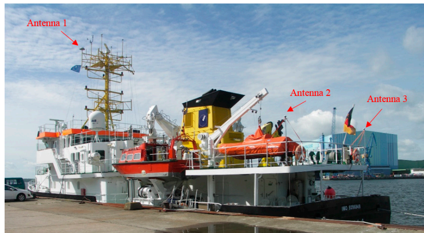
Figure 1. The ship used in the Baltic Sea gravimetric campaign and the positions of the three Global Navigation Satellite System (GNSS) receiving antennas.
