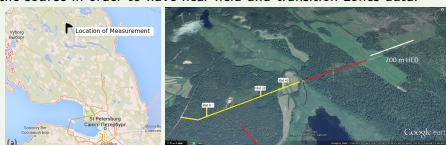
Fig. 4 : (a) Location of measurement in Vuoksa region, Russia. (b) Previous RMT field survey profile and far field zone (yellow), CSRMT profile (yellow + red) and 700 m HED (white), station 8, 31 and 44 are marked for 1D inversion.
