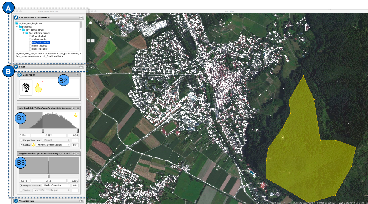
Figure 2: Visual interface of our approach. The spatial distribution of PS points in the Stauffen area after applying two filters is depicted in a map. Various filters can be defined and combined in the configuration and filter component (left). It comprises a list of available parameters (A), a filter panel (B), and a visualization panel (not shown). Parameters for filtering are selected by dragging and dropping them from A into B. In this example, the filter criteria are the temporal coherence (B1) and the relative point height (B3). The minimum threshold for the coherence is determined by the maximum coherence value of the (now excluded) points in the polygon (see map and geography library B2).
