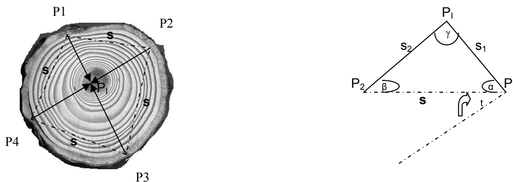
Figure 3: Cross section with ring measurements indicated (arrows, left side) and trigonometric parameters to calculate the intersection point P_1 (right side).
