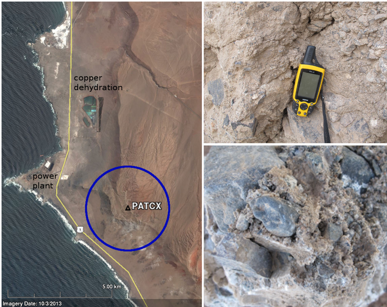
Figure 4. Map of the surroundings of station PATCX. The station is located at an altitude of 830 m. The next paved road has a minimal distance of 2.6 km. A power plant is located on the peninsula at a distance of 4.3 km and a copper dehydration plant is located 4.8 km NNW. The blue circle illustrates the region of sensitivity for the autocorrelations (see Section 3.1). The material at the station, a conglomerate, is shown at the right. (Map: Google, map data: NNES/Astrium, Digital Globe; pictures: B. Schurr).
