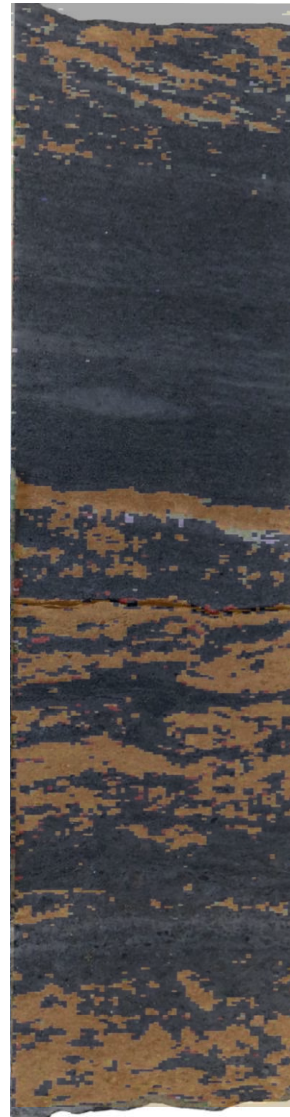
Figure 35: Classified minerals after MICA algorithm based on the hyperspectral data on sample 689.
