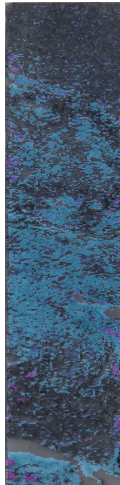
Figure 37: Classified Fe-bearing minerals based on the hyperspectral data on sample 625.
