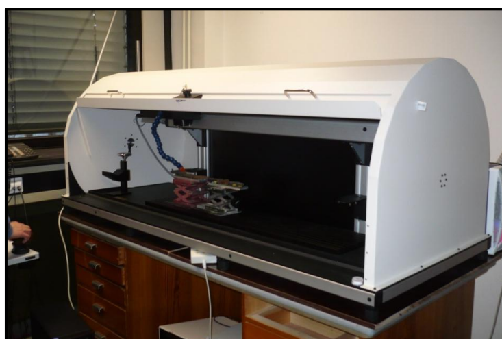
Figure 12: LIBS drill core scanner in Hannover. (Photo by Jeannette Meima)
