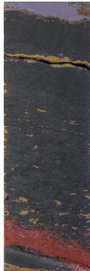
Figure 33: Classified minerals determined using MICA algorithm based on the hyperspectral data on sample 550.
