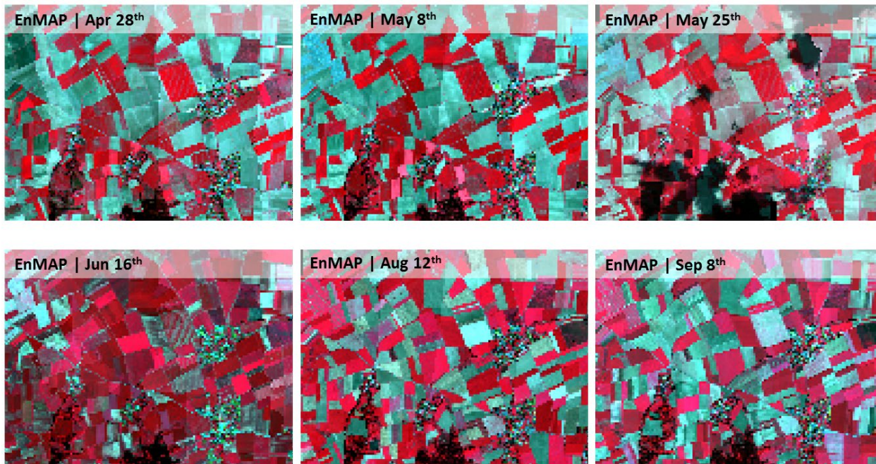
Figure 3.01: Artificial EnMAP image time series derived from the multisensoral airborne hyperspectral image series recorded from April 28 th to September 8 th 2012 over the Neusling test site in southern Germany.
