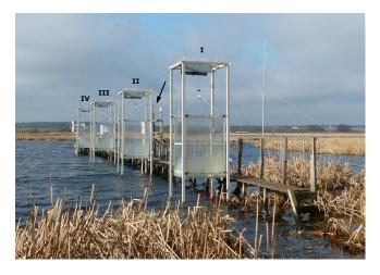
**Figure 1.** Transect of automatic chambers (ACs) established at the measurement site. The arrow indicates the position of the climate station near chamber II.
