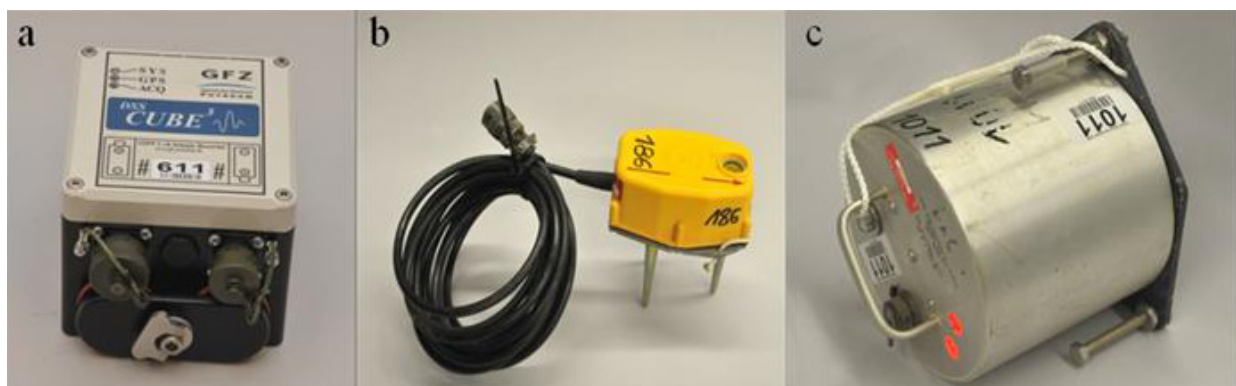
Figure 2. Short-period seismic stations deployed on-land during the experiment and belonging to the GIPP (Germany). (a) DATA-CUBE3 recorder; (b) 3-D PE-6/B Geophone; (c) Mark L4C sensors.
