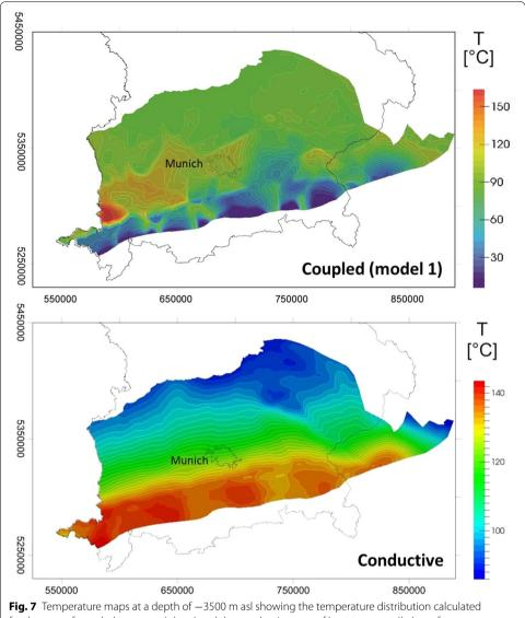
**Fig. 7** Temperature maps at a depth of -3500 m asl showing the temperature distribution calculated for the case of coupled transport (*above*) and the conductive case of heat transport (*below*, after Przybycin et al. 2015b)
