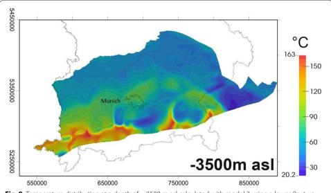
**Fig. 9** Temperature distribution at a depth of -3500 m as calculated with model 2 using a lower (by two orders of magnitude) hydraulic conductivity of the Folded Molasse Sediments compared to model 1
