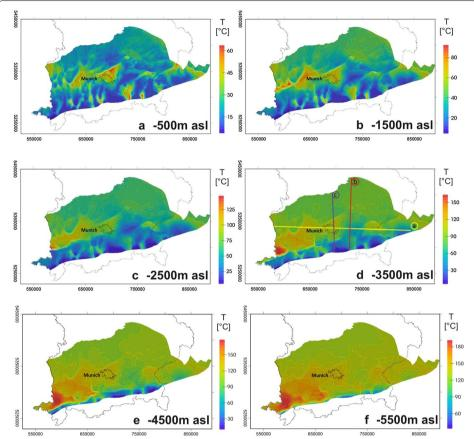
**Fig. 6** Predicted temperatures by the coupled fluid flow and heat transport simulations without considering faults in the system (model 1). The model predicts widespread negative thermal anomalies (*blue colours*) at shallower depths (maps **a** and **b**). The small positive thermal anomalies (*reddish colours*) from shallower depths increase in size with increasing depth (maps **c-f**). Profile lines are depicted in map **d** for which the temperature distribution is shown in Fig. 8
