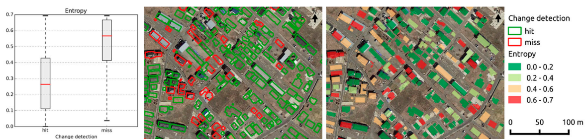
Figure 12. Relation between change detection performance (hits and misses) and classifier confidence (entropy).
