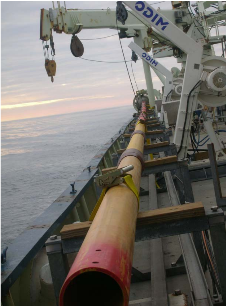
982 Fig 1. The Long Piston Corer of Woods Hole Oceanographical Institution. The thick- 983 walled steel core barrels are held together by joints. The core shoe and the core catcher 984 are removed to allow inserting a liner. The large weight set is in the back. (Foto: 985 Kallmeyer, GFZ)
