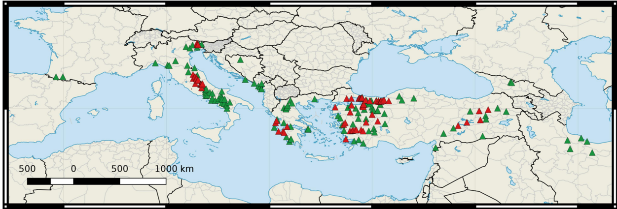
Fig. 4 - Distribution of sites for ergodic and region-specific PSHA (green), sites with 5 or more recordings for site-specific PSHA (red) in the RESORCE dataset
