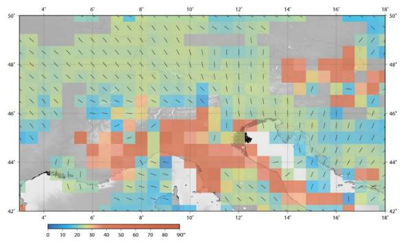
Fig. 11: Visualization of mean S<sub>Hmax</sub> orientation and variance.
