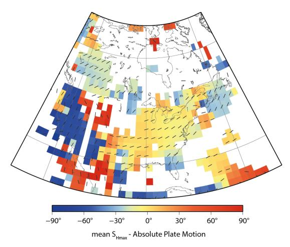
Fig. 10: Deviation between absolute plate motion direction and mean  $S_{Hmax}$  orientation. The difference between the mean  $S_{Hmax}$  orienation and the absolute plate motion direction is presented by colour coded patches on a 1° grid with the mean  $S_{Hmax}$  orientation on a 2.5° grid displayed by lines.
