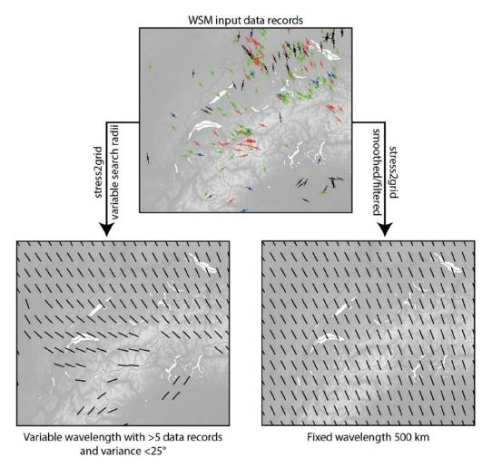
Fig. 2: From stress data records to mean  $S_{Hmax}$  orientation on a regular grid. Top: Stress map with data records from the Western Alps. Bottom: The *Stress2Grid* script derives a smoothed mean  $S_{Hmax}$  orientation with a fixed search radius of 500 km (right) and a mean  $S_{Hmax}$  orienation using different search radii and variance threshold of < 25°
