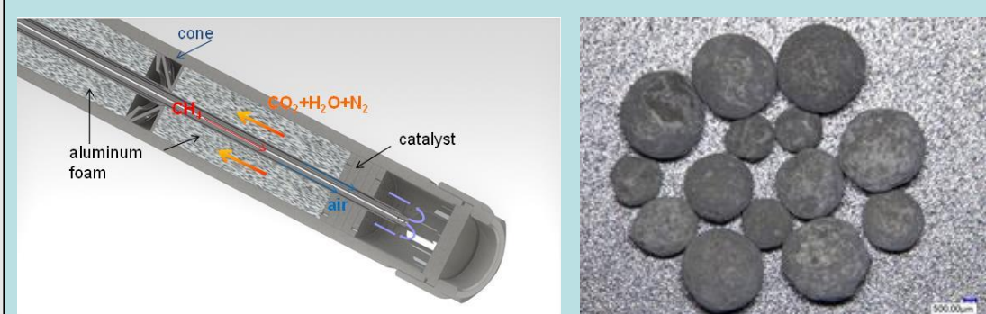
Figure 6: Technical sketch of the counter-current heat-exchange reactor.
