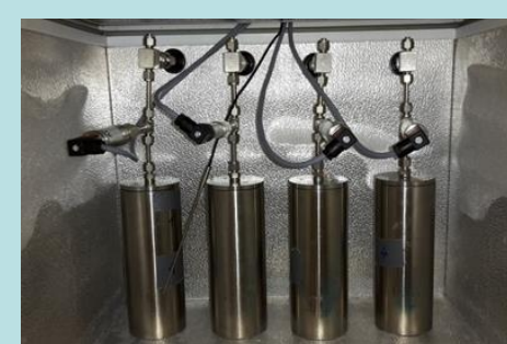
Figure 4: pressure vessels equipped with p-sensor stored in cooling box.
