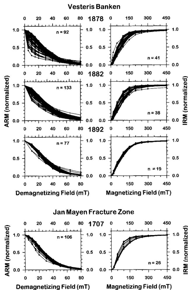
**Figure 1.** Normalized demagnetization curves of the anhysteretic remanent magnetization (ARM) and acquisition curves of the isothermal remanent magnetization (IRM) from the cores investigated. The IRM curves are normalized to the saturated IRM acquired at 1500 mT, defined as SIRM. For reasons of clarity the plots are cut off at 450 mT because all recorded curves reach saturation between 450 and 1000 mT. *n* denotes the number of samples investigated.
