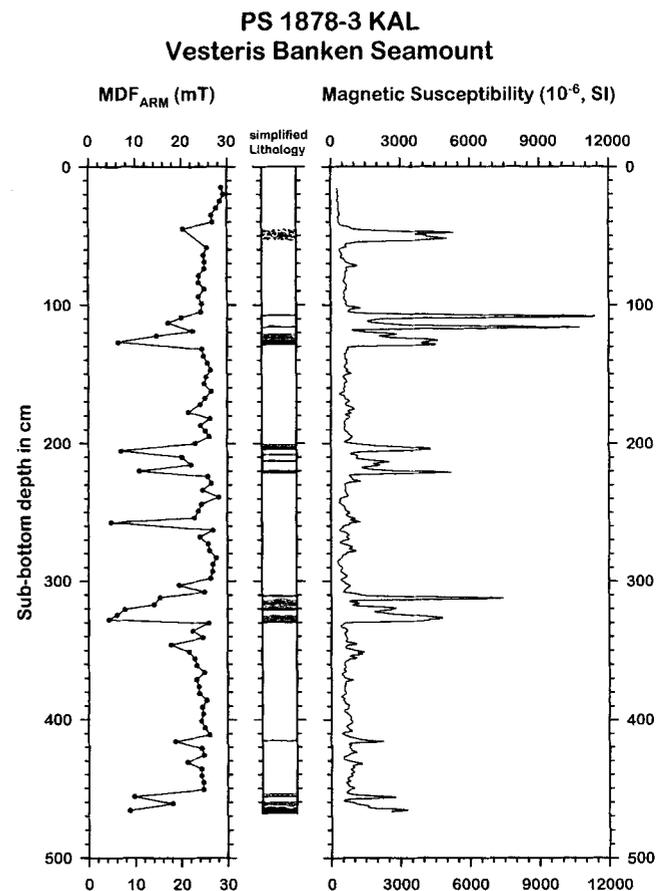
**Figure 2.** Core PS 1878-3 KAL: downcore variations of the median destructive field (MDF) of the anhysteretic remanent magnetization (ARM) (left), simplified lithology (middle) and high-resolution log of magnetic susceptibility (right). Extremely high susceptibilities as well as low MDF<sub>ARM</sub> values correspond to coarse-grained volcanic ash layers indicated by grey and black stripes in the lithology log.
