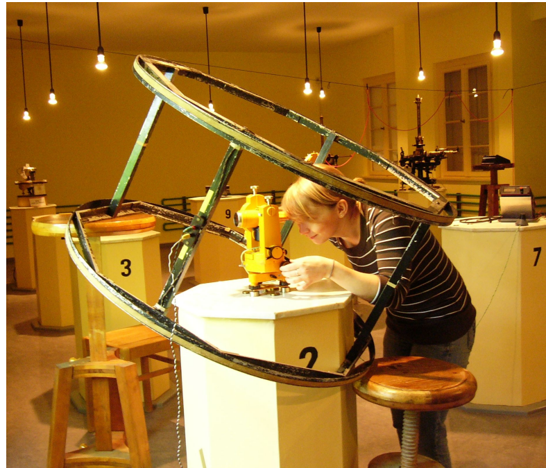
Figure 2.11: An artificial field gradient has been applied on the DI3 instrument by using a Helmholtz system with opposite connected rings. The field gradient leads to differences at the sensor positions drawn on the right side.
