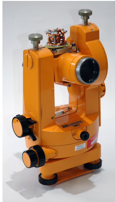
Figure 2.8: The DI3 instrument: A Zeiss theodolite equipped with a three component fluxgate sensor.
