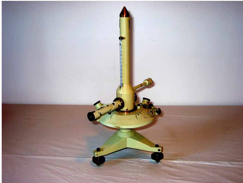
Figure 2.3: A Quartz Horizontal Magnetometer. The vertical tube houses the quartz fibre, the twisted magnet can be observed through the horizontal tubes. The foot screws allow for the levelling of the instrument. Courtesy: Geological Survey of Canada.
