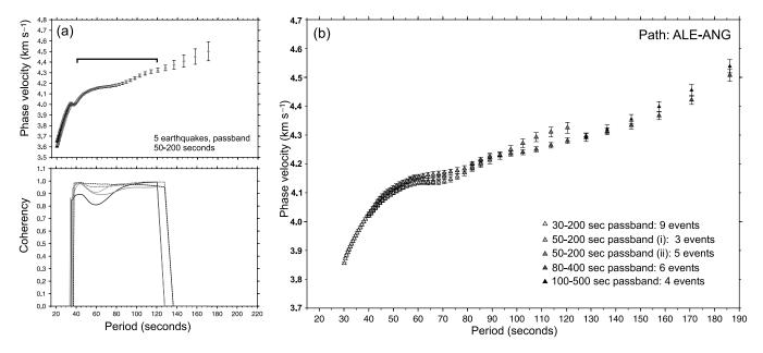
Figure 5. (a) Example of dispersion curve computed for five earthquakes in the 50–200 s passband, for path ALE–ANG. Top: dispersion curve with error bars. The horizontal bar indicates where the results are well resolved and reliable. Bottom: waveform coherencies for the five earthquake pairs used in the analysis. (b) Composite dispersion curve for path ALE–ANG, composed of reliable results from several different passbands using several seismogram pairs in each case.
