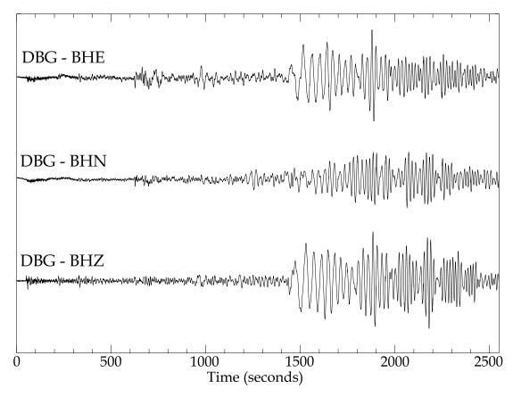
**Figure 3.** An example of the teleseismic data used in this study. The figure shows the three-component seismogram set (BHE, BHN, BHZ) for the 2000 July 21 ( $M_{\rm S}$  6.1) Costa Rica earthquake, recorded by station DBG. The backazimuth of the earthquake from the station is 248° and the epicentral distance is 74°. Rayleigh waves on the vertical component seismogram clearly show their dispersive nature.
