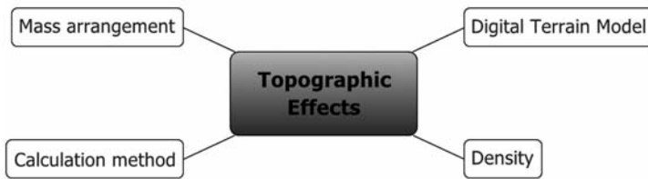
Figure 2: Input data and modelling parameters for the calculation of topographic effects
