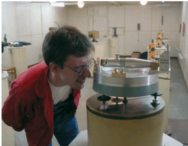
Fig. 4: Orienting a first prototype of an instrument under development at Niemeck observatory. This instrument eventually will allow for the automatic absolute determination of three field components.
