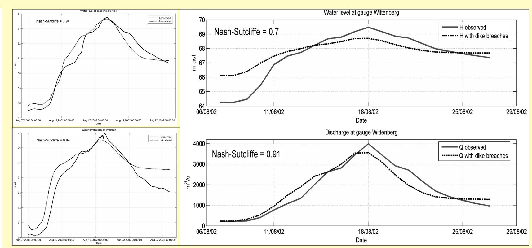
Figure 5. Comparison of water level and flow hydrographs
