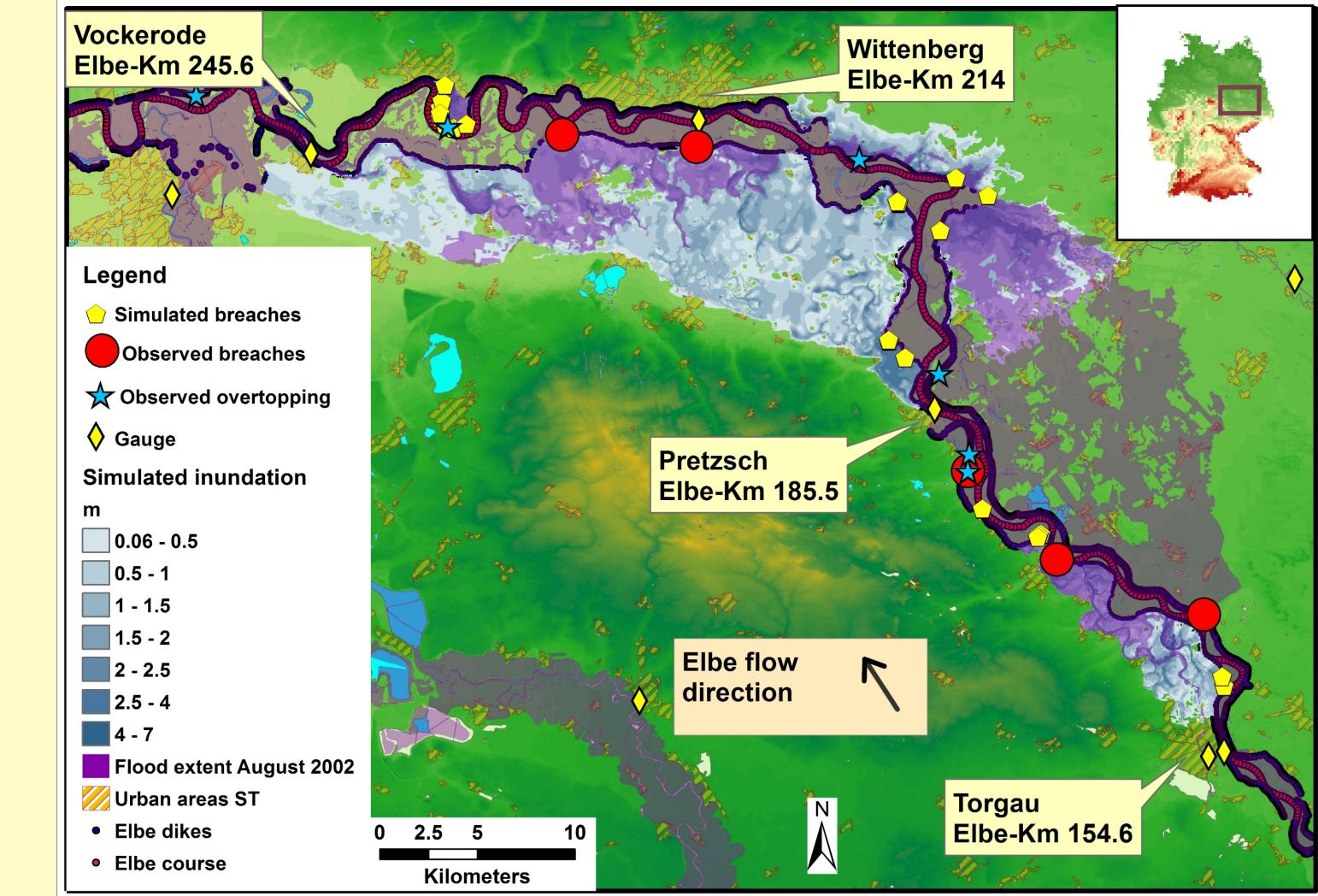
Figure 4. Maximum simulated inundation (Flood area index F = 25.2 %)
