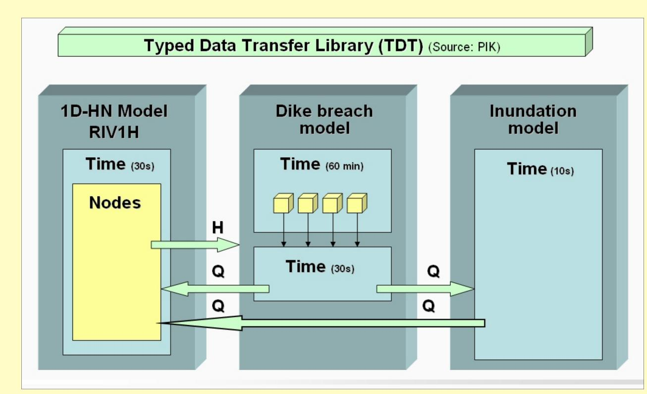
Figure 3: Schematical representation of the coupled models and exchange variables H (water level) and Q (discharge). The time iteration loops are given exemplarily and can be changed by the user.
