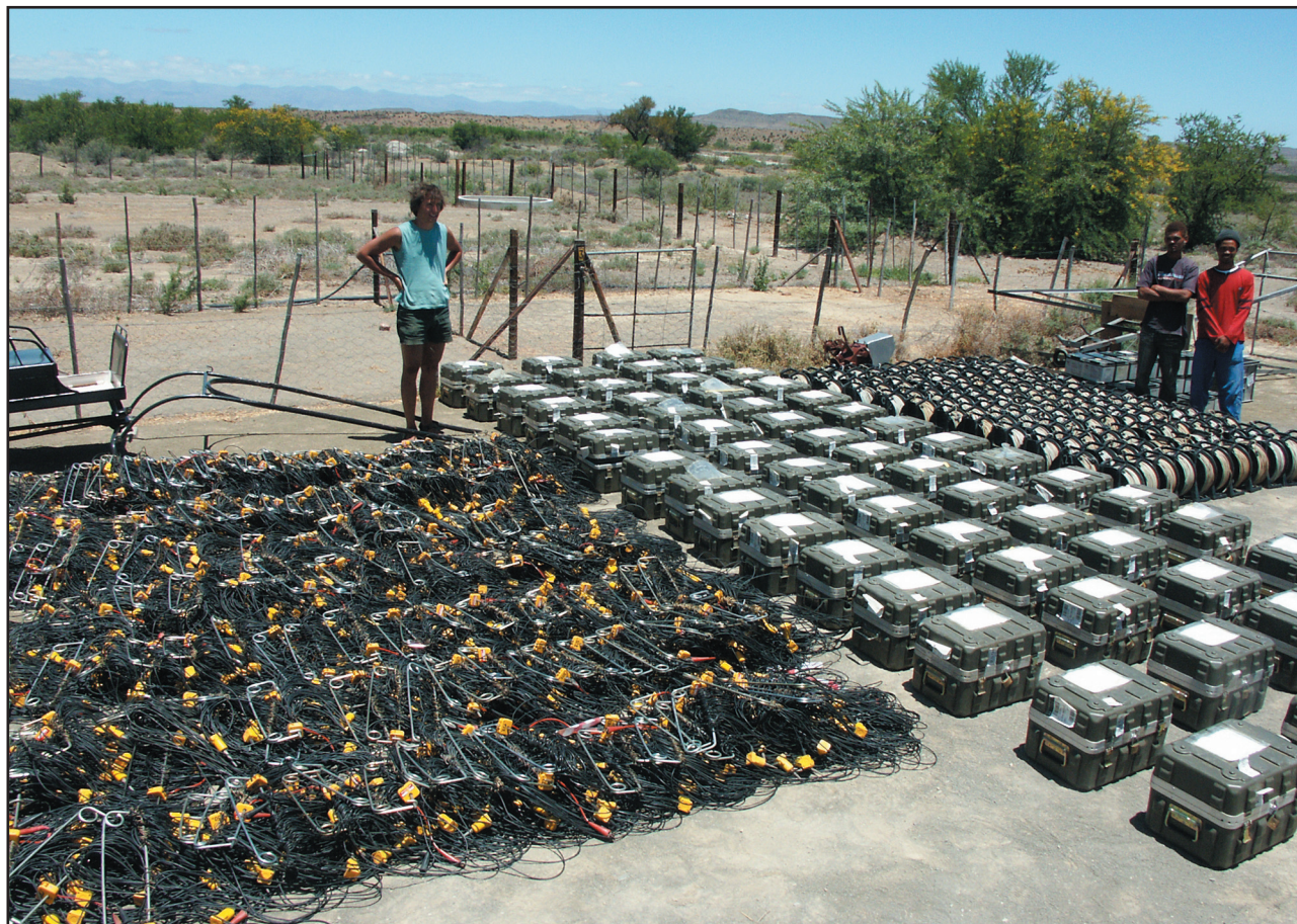
Figure 4. (c) geophysical instruments from the Geophysical Instrument Pool, Potsdam. From left to right: geophone strings, recorders, cables and batteries. Detailed parameters of the instruments and deployment technique are listed in Table 2.
