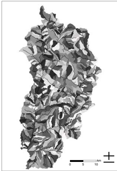
Fig. 3: Example of a delineation of a catchment into 660 elementary hillslope areas (Ésera basin, North-Eastern Spain, basin area: 1231 km 2 )
