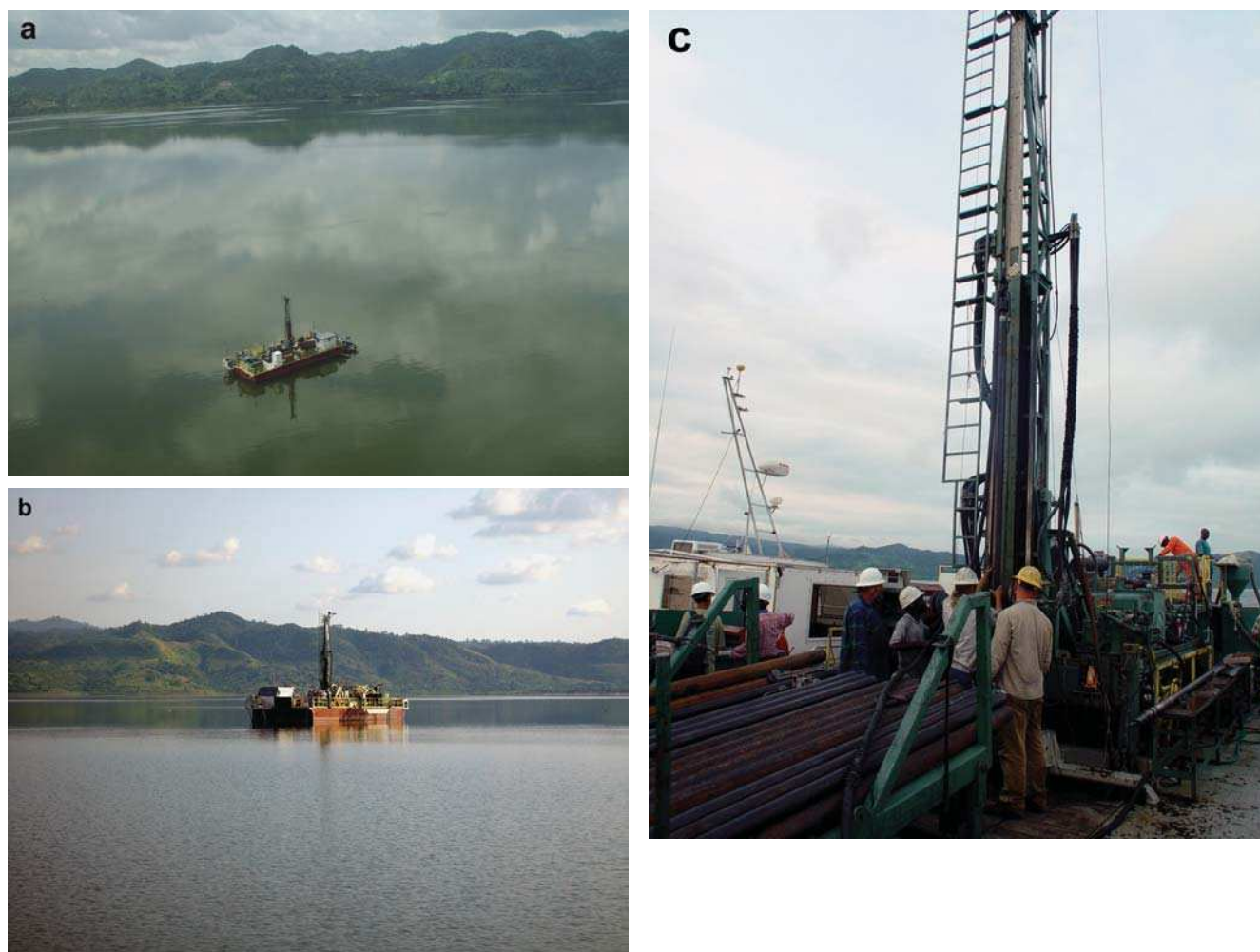
Fig. 11. Views of the GLAD800 drilling barge and rig. a) An aerial view of the drilling barge on Lake Bosumtwi. b) The GLAD800 on the lake, showing the floating containers on which the drill rig is mounted. c) A close-up of the modified Christensen CS-1500 diamond coring rig mounted on the barge. All images: C. Koeberl.
